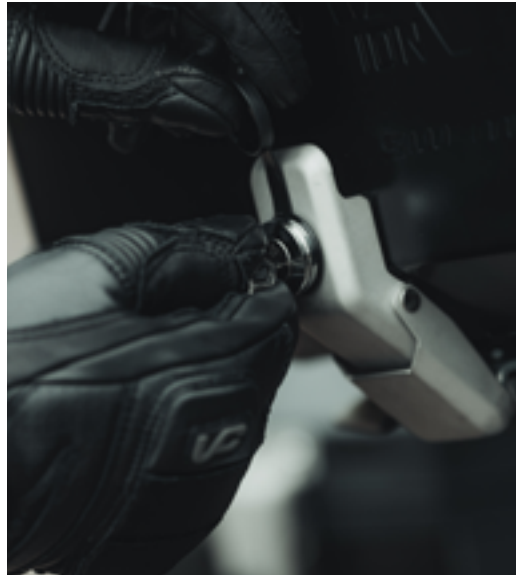
A lock in the latch buckle secures the top case against theft.
