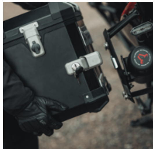
The side cases can be easily clipped into the four retaining cams on the carrier.
