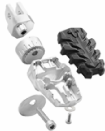
The individual components of the EVO footrest.
