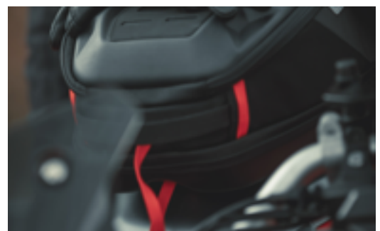
The tank bag is detached from the tank ring using the pull cord
