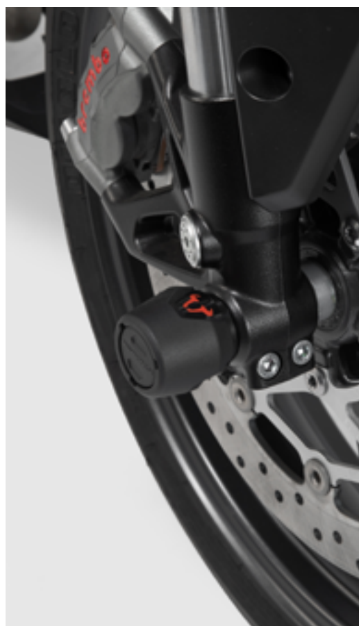
Glass fiber-reinforced plastic with damping TPE coating.
