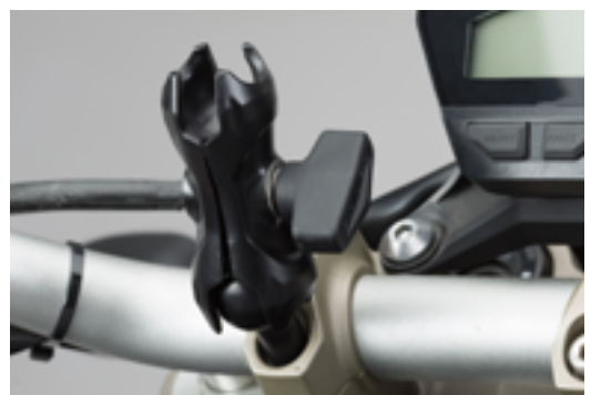
Swiveling clamp arm on the 1" ball holder.
