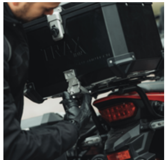
The latch buckle lets you quickly and securely attach your top case.
